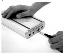
1. Do not connect AC Adapter to the enclosure. unscrew to loosen the Back Panel and remove the Back Panel from the Enclosure.
